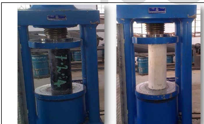
Fig 4 Compression strength test of concrete specimen confined with HDPE and UPVC Pipe.
