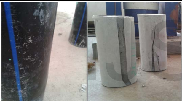
Fig 5 Failure of HDPE and PVC Confined Concrete specimen
